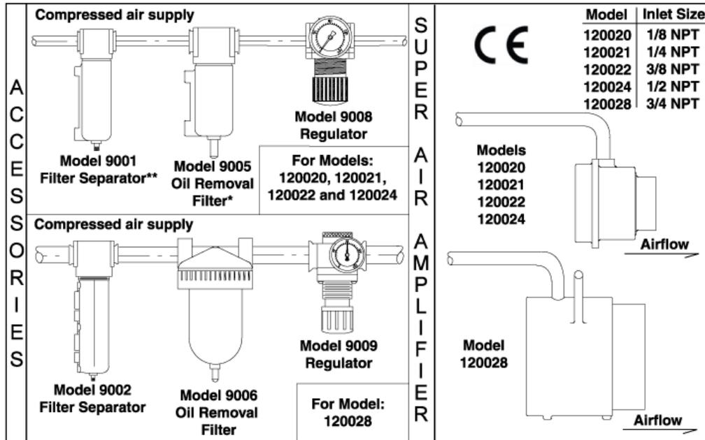
\*For Model 120024 and 120028 Super Air Amplifier - Use Model 9006 Oil Removal Filter
